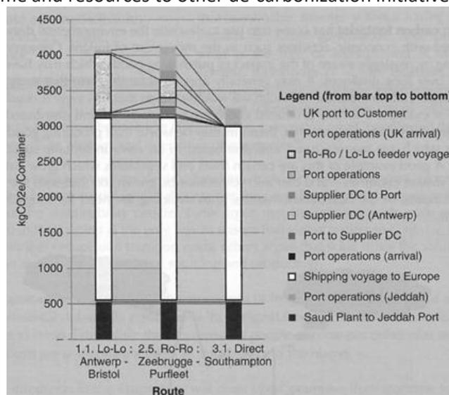
**Figure 6.** Carbon footprint for a container journey (three alternative routings).
